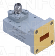
42WCAK_Cu Right Angle Rectangular Waveguide to Coaxial Adapter 18-26.5GHz WR42 to 2.92mm Female
